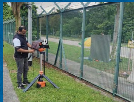
PVAIDS portable camera being redeployed and set up at a new location to mitigate increased intrusion risk from nearby construction.
